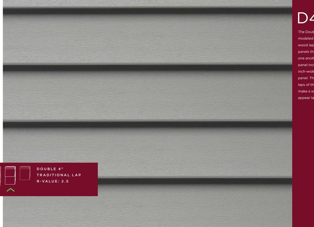
The Double 4" style is modeled on traditional wood lap siding with panels that overlap one another. Each D4 panel includes two fourinch-wide laps on each panel. The narrower laps of the D4 panel can make a smaller home appear larger.
