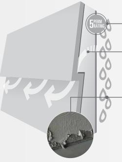
The EPS foam backing has a Permeability Rating of 5.
